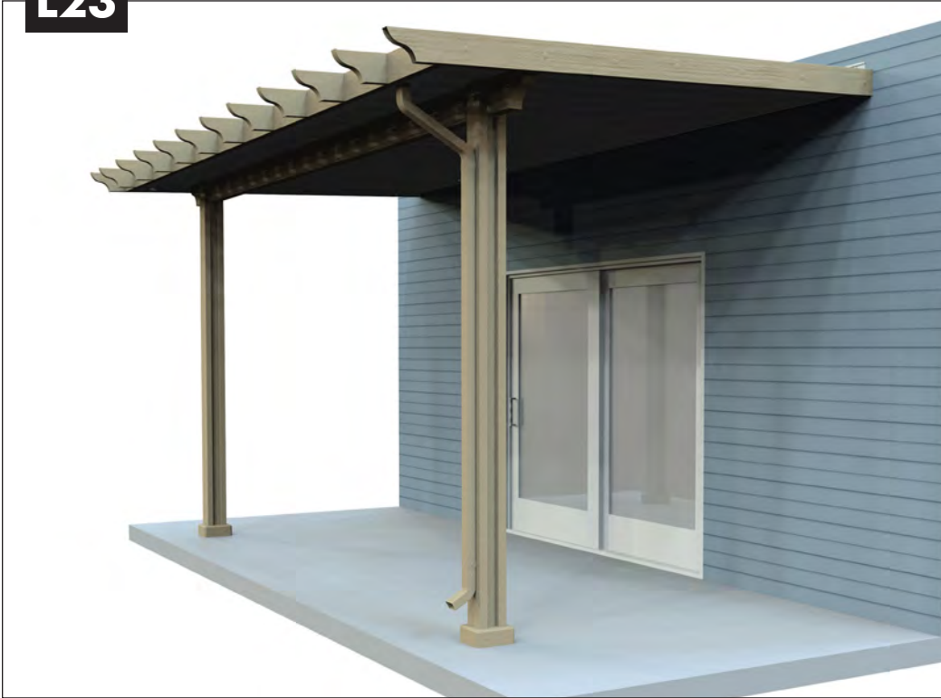
L23. Finished patio cover with lattice wrap.
